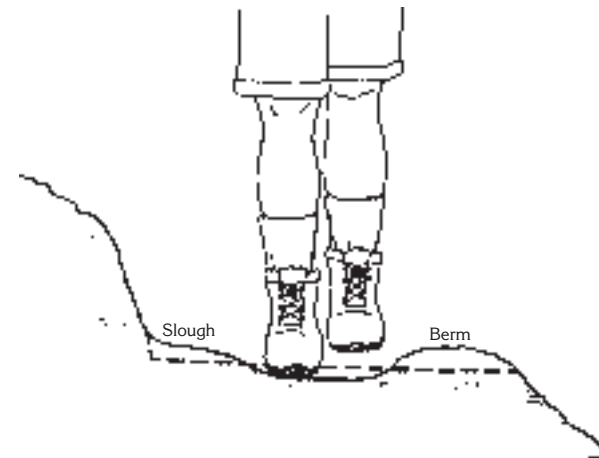
Figure 17—Remove the slough and berm, leaving the trail outsloped so water will run off. One fist's worth of drop for the length of a Pulaski is a good rule of thumb.
